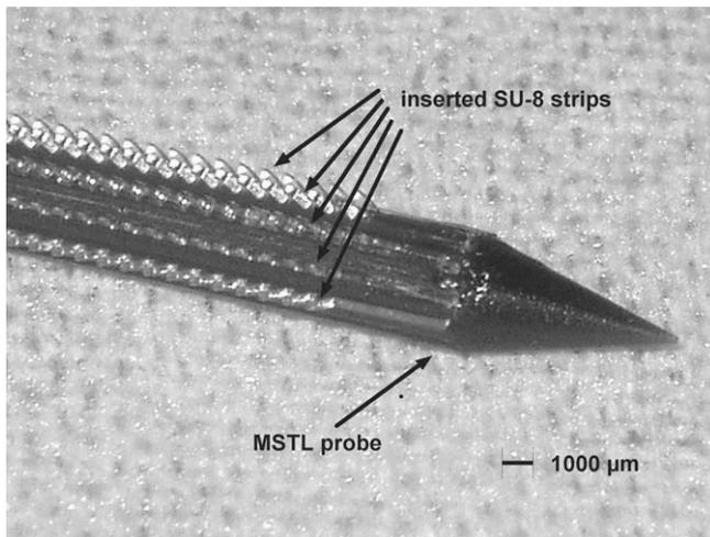
Fig. 4. Assembled MSTL probe with 12 SU-8 strips (fins protruding 500 μm from surface).
