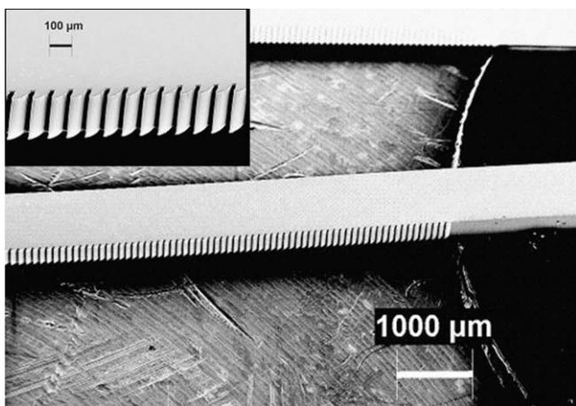
Fig. 2. Individual strip with HAR microstructures on the side wall made from SU-8 photoresist; inset shows detail of the fin structures.
