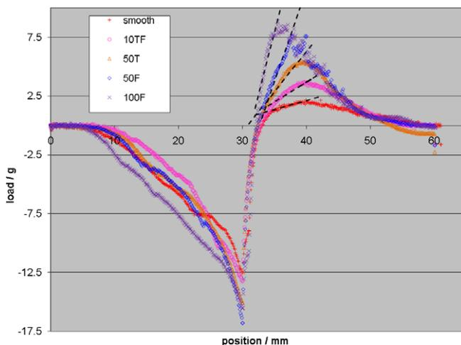
Fig. 5. Load–displacement diagram for insertion and retraction of assemble probe into brain tissue; dotted lines indicating linear increase of load during probe retraction.
