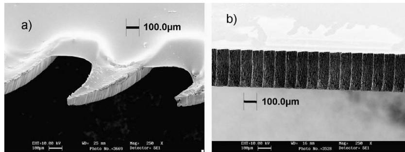
Fig. 3. (a) Silicone microstructure; (b) Si microstructure.
